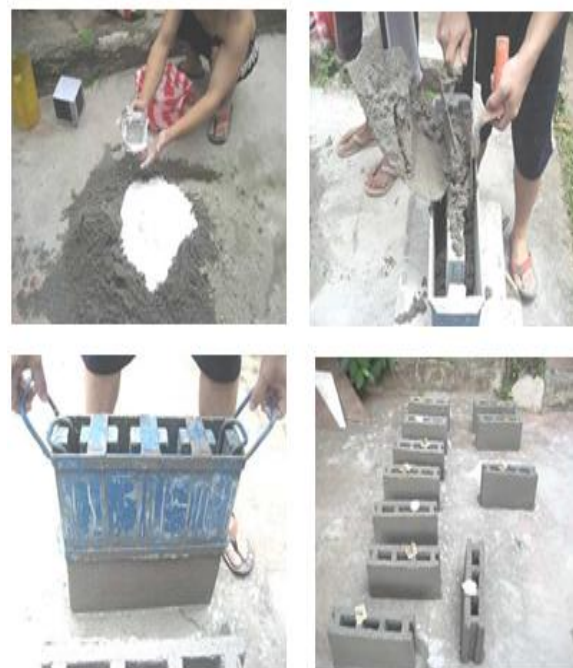
Fig. 6. Making of concrete hollow blocks with sieved; recycled flat window glass
