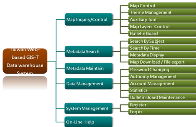
Fig. 5. Function design of the proposed web-based GIS-T data warehouse system.
